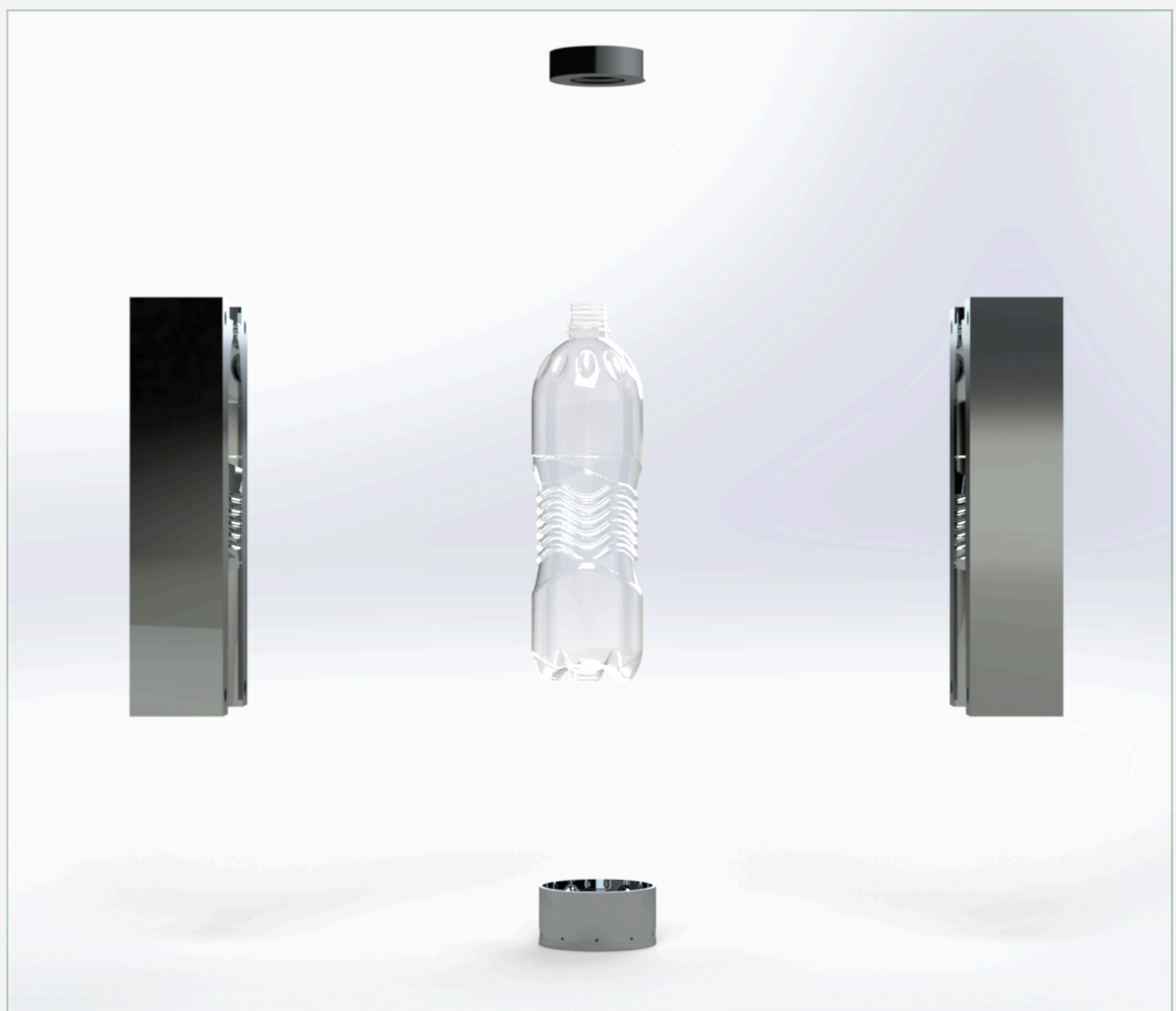
3D Design of the bottle and its mold (Figure 10.2)
