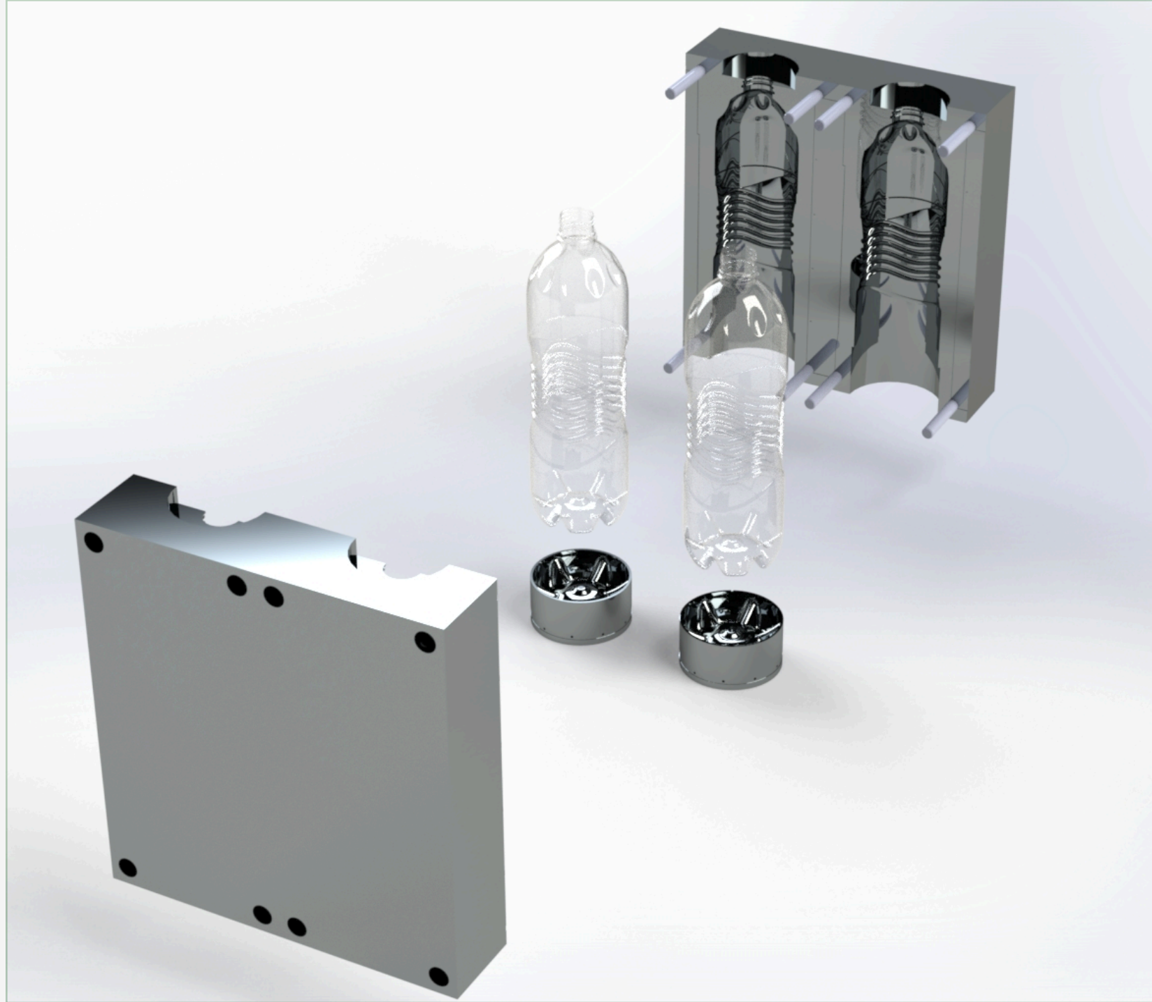
3D Design of the bottle and its mold (Figure 10.1)
